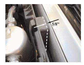
Due to the larger 57mm core, the stock shroud must be trimmed 5/8".
